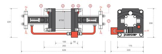
Type : GB-DS type PI – Air driven Inlet Pa – Inlet Pb – Outlet
