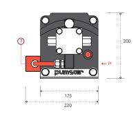
Type : GB-SS type Pl – Air driven Inlet Pa – Inlet Pb – Outlet
